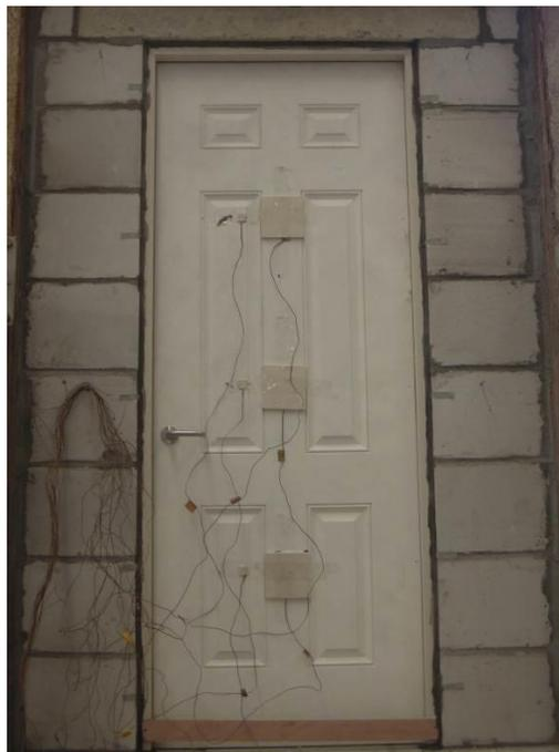
Fig. 2 Unexposed Side Prior to the Fire Test
