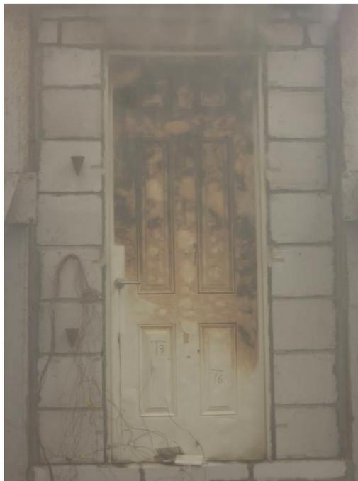
Fig. 4 Unexposed Side after 16 Minutes
