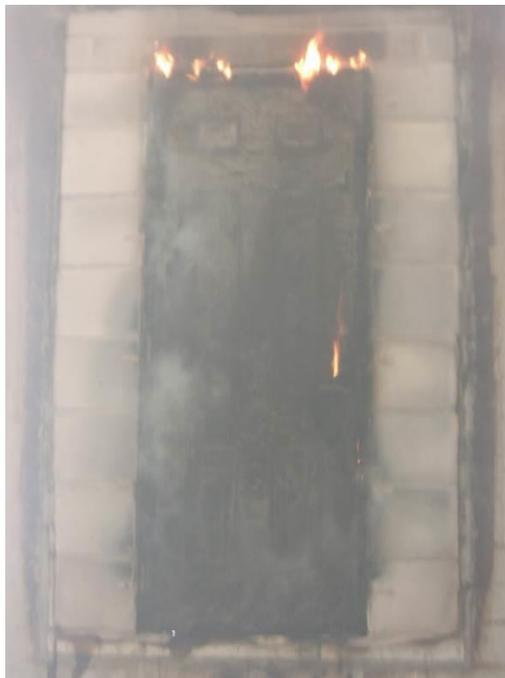
Fig. 6 Exposed Side after 20 Minutes
