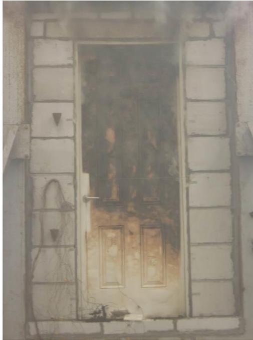
Fig. 5 Unexposed Side after 20 Minutes
