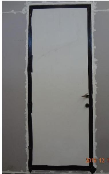
Fig. 1 Unexposed Side of outswing test door assembly during air leakage test
