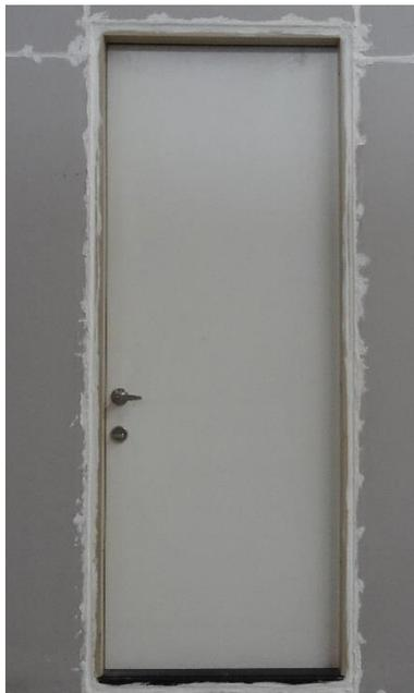
Fig. 2 Unexposed Side of inswing test door assembly during air leakage test
